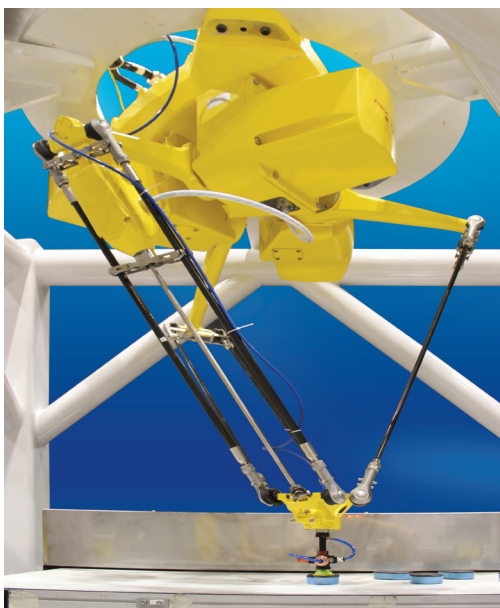
Food picking with four-axis M-2iA/3SL
